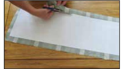
3. When complete and inspected, cut off surplus covering by running a sharp knife all round the edges of the panel or use scissors.
