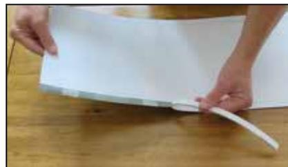
5. Carefully, to avoid fraying, remove the broken strips of PVC to leave your covering's edge.
