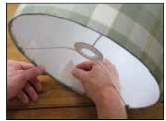
**16.** Use the finishing tool to push the fabric behind the rings. Force the tool between the gap and swipe around the circumference until you're happy with the finish.
