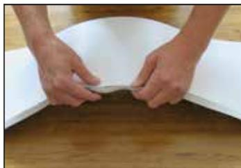
4. Snap back the creased edges (kiss cut) around the panel to break the edge of the PVC.
