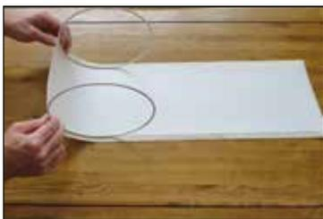
**20.** Roll the rings onto the panel keep the rings in-line with the PVC edge at all times, steps 11,12.
