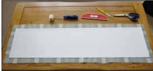
1. Cut down your covering to a workable size. Place face down and position the large panel on top and make sure it fits within covering.
