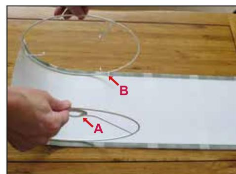
11. Place the rings on the PVC edge and start to roll towards the seam edge (Pic 7).
