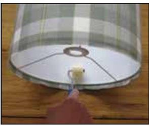
**13.** Turn over so the seam is now on a hard surface and apply firm pressure pressing the tape down with your hand or use a seam roller.
