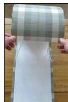
12. Roll towards you and keep the rings in-line with the PVC edge at all times. If you run out of line simply go back and correct.
