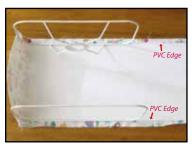
**15.** Keep frame in line with the PVC edge at all times. If you run out of line go back and correct.
