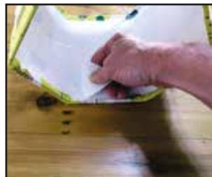
**23.** Use the finishing tool to push the fabric behind the frames.
