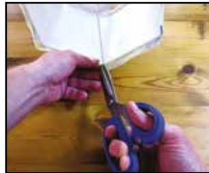
**20.** Snip the covering in line with the struts on the utility frame so that the covering can be folded behind.
