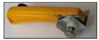
The creasing tool is used for putting a score (kiss-cut) at a set distance from the edge of a lampshade panel. After the cut has been made you can snap back the score line to break the PVC and remove the PVC strip leaving a fabric edge to roll behind the lampshade frame.
