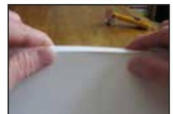
**When complete snap back the crease line to break the PVC edge and remove.**
