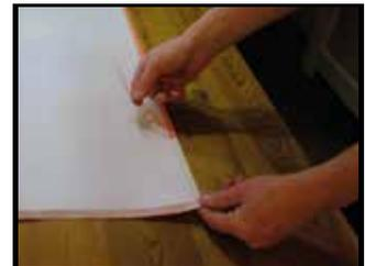
9. Remove the release paper and your panel is now complete and ready for attaching to the frame.
