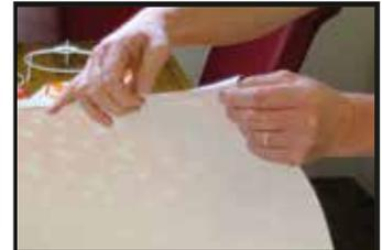
6. Snap back the creased edges (kiss cut) around the panel to break the edge of the PVC.
